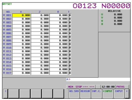
Fig. 2.1.1 (c) With tool wear offset
